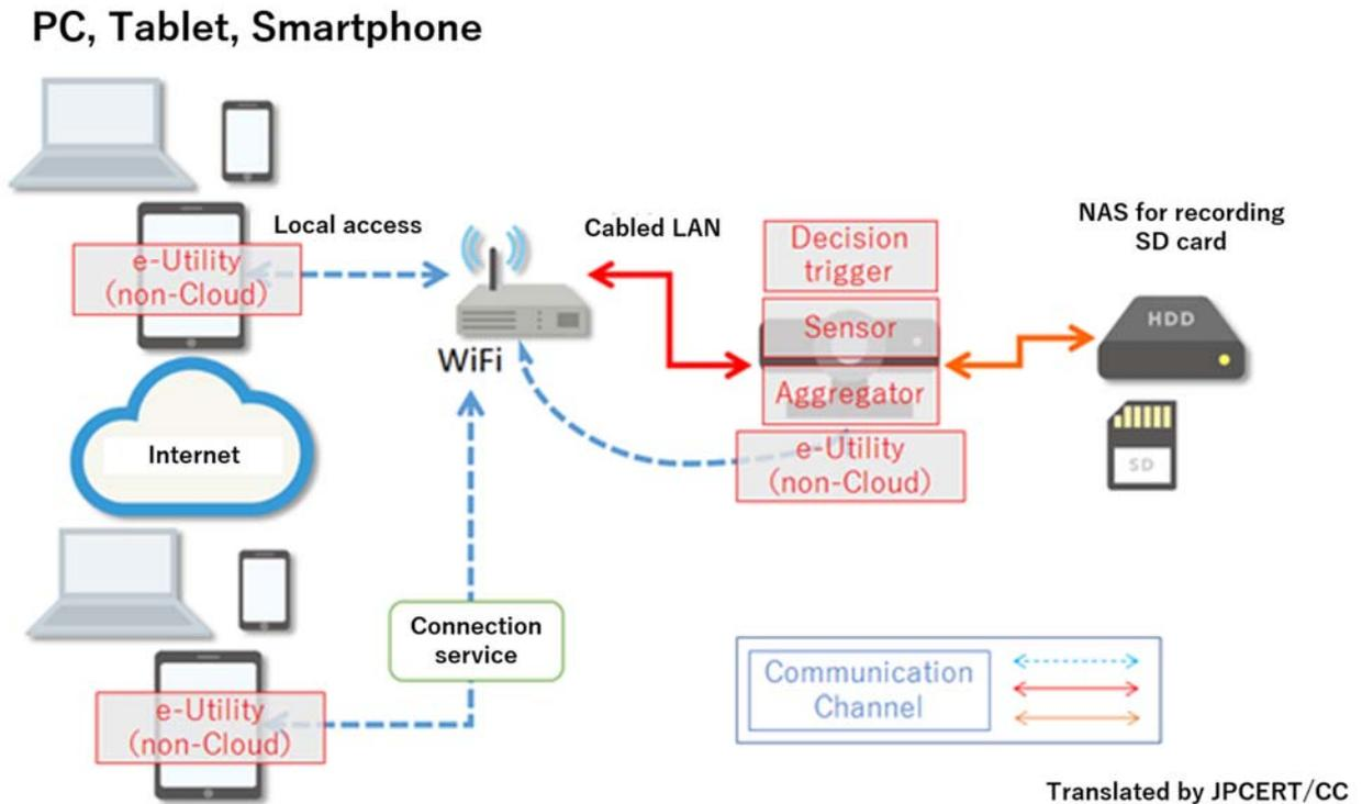
[Figure 5 Categorization by primitive in the case of a network camera]
