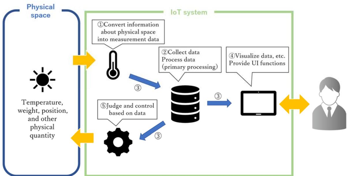
[Figure 1: How IoT systems operate]
