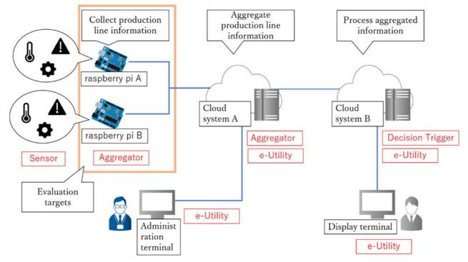
[Figure 3 Production information collection system in a factory]
