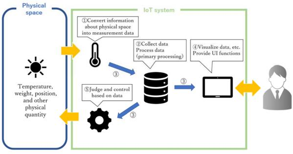
[Figure 1: How IoT systems operate]
