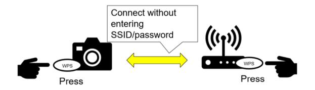
Developer: Consider security when providing a WPS function (e.g., MAC address filtering) User: Check that WPS functions properly
