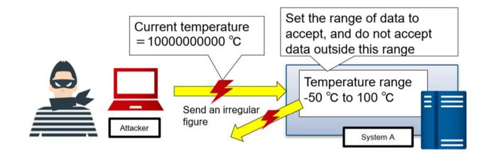
Developer: Provide a function for restricting data to be accepted
