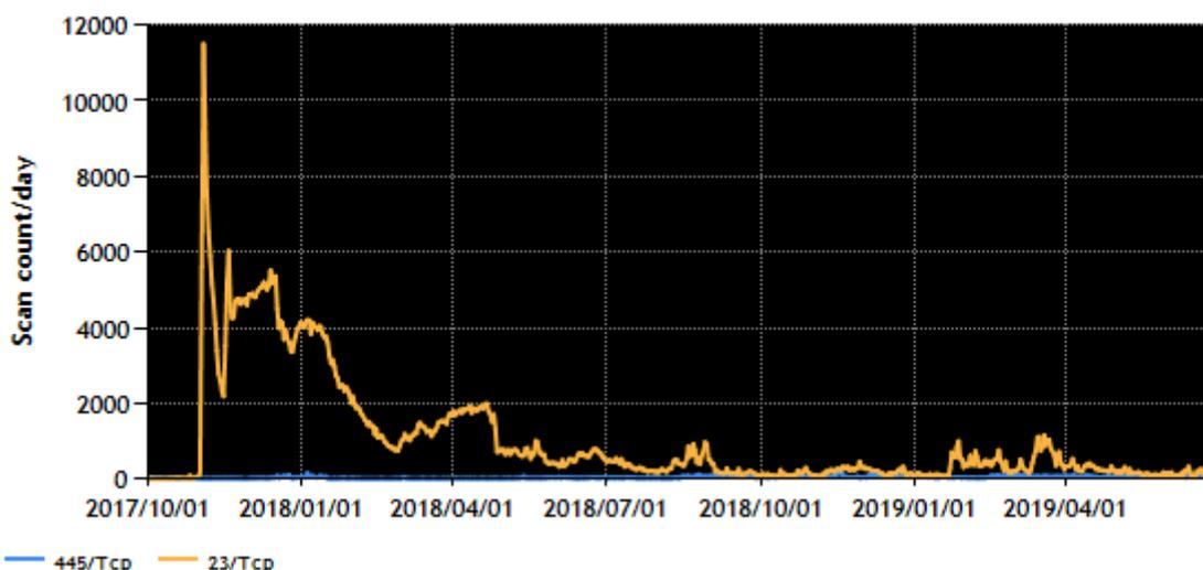
[Figure 4: Long-term trend in numbers of packets targeted to port 23/TCP and port 445/TCP]
